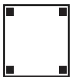
Placing the subwoofer in the corners usually gives much amount of bass but with less precision and definition.
