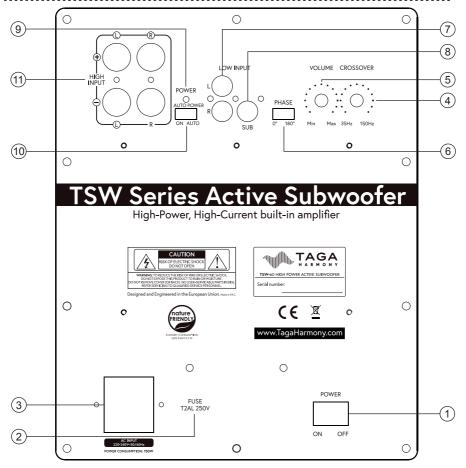
Available controls and inputs as well as their placement on the rear panel may vary depending on the model. The above figure shows the TSW-60 subwoofer rear panel.
