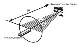
Use the remote controller by aiming it at the remote controller sensor. The remote controller can operate in the maximum range of 5 meters away from the amplifier and within 30 degrees from the axis of the controller sensor.
