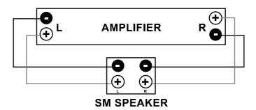
If your speaker is wired incorrectly it will be out of phase and it will sound indistinctly and with a weak bass. Re-check your connections and correct the polarity by reversing the connections.
