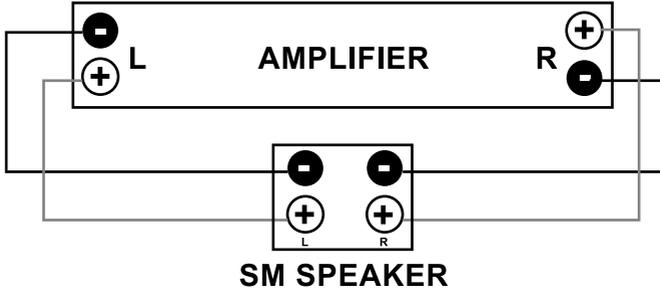
If your speaker is wired incorrectly it will be out of phase and it will sound indistinctly and with a weak bass. Re-check your connections and correct the polarity by reversing the connections.
